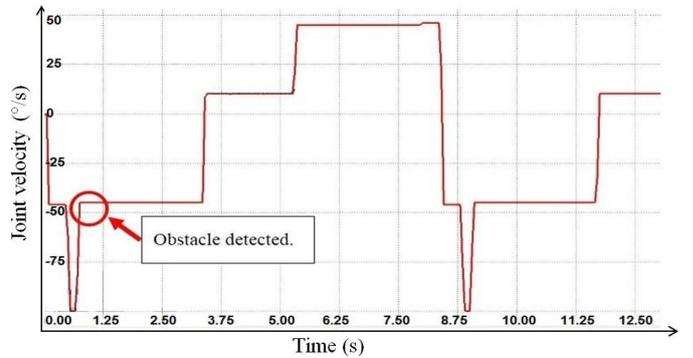
Figure 12: Joint 1 angular velocity in ‘limit speed’ mode
