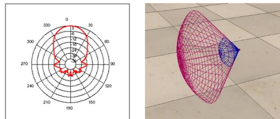
Figure 2: (Left) Conical beam pattern; (Right) Cone type proximity sensor
