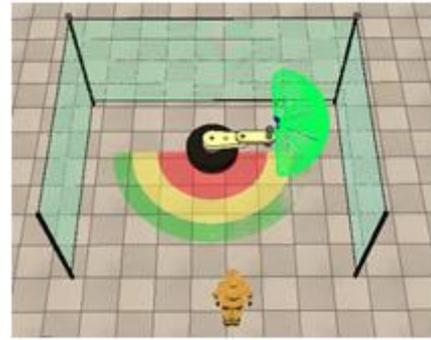
Figure 6: Illustration of the reach of the robot and the direction of the approaching human
