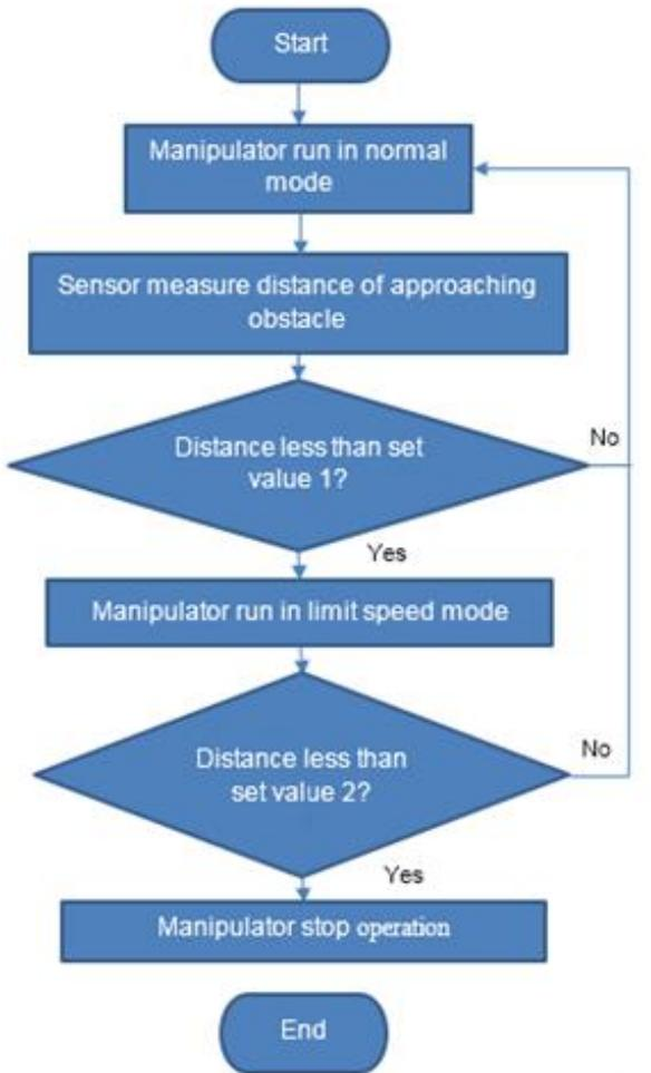
Figure 4: System flow chart of the collision avoidance strategy
