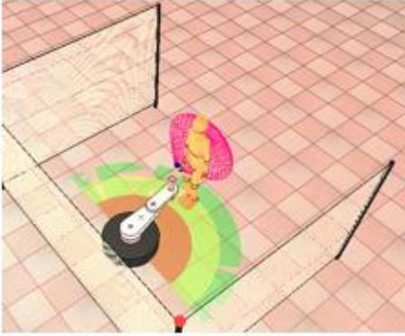
Figure 14: Illustration of 'stop' mode
