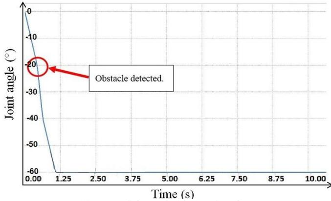
Figure 15: Joint angle 1 in 'stop' mode
