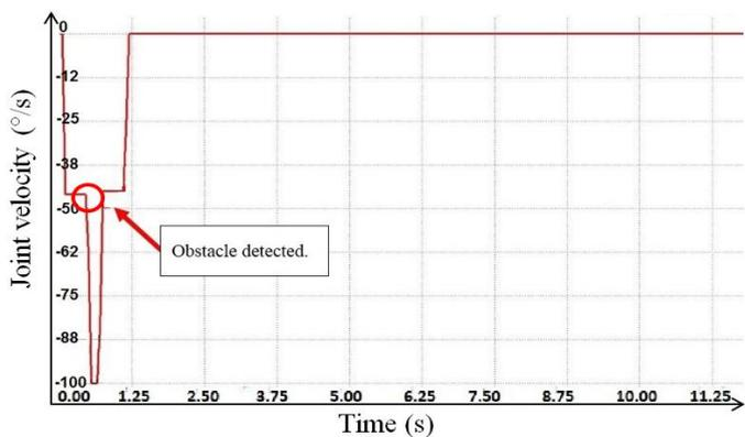
Figure 16: Joint angle 1 velocity in 'stop' mode
