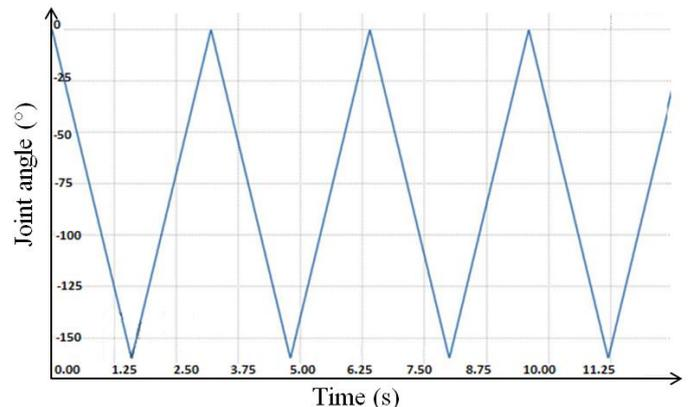
Figure 7: Joint angle 1 of the manipulator in normal mode (no obstacle)
