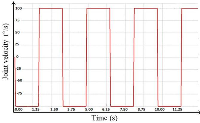
Figure 8: Joint 1 angular velocity in normal mode
