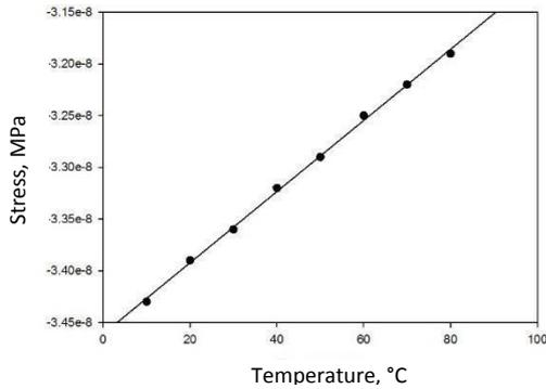
Figure 3: Temperature versus silicon dioxide film stress
