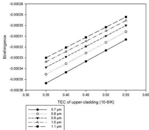
Figure 7: Birefringence versus thickness of upper-cladding and TEC
