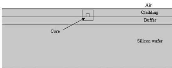
Figure 1: Schematic model of planar waveguide
