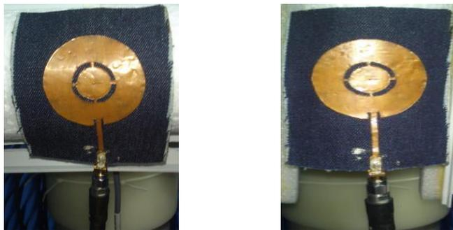
(a) E-plane bending (b) H-plane bending
