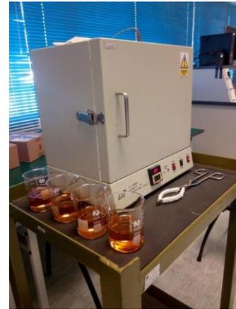
Figure 5: Lab oven used to heat oil
