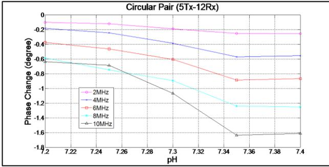
Figure 2: Result of phase change for Circular Pair (5Tx-12Rx)
