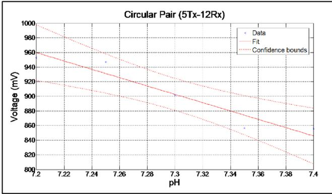
Figure 6. Linear regression for circular coil pair (5Tx-12Rx)
