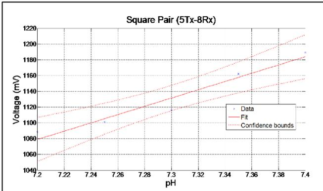
Figure 7. Linear regression for square coil pair (5Tx-8Rx)
