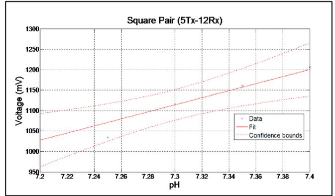
Figure 8. Linear regression for square coil pair (5Tx-12Rx)
