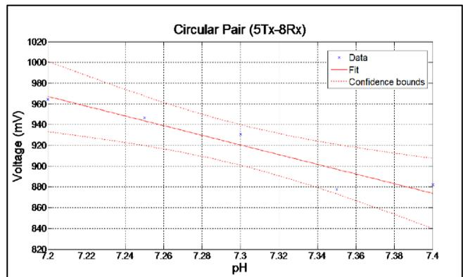
Figure 5. Linear regression for circular coil pair (5Tx-8Rx)
