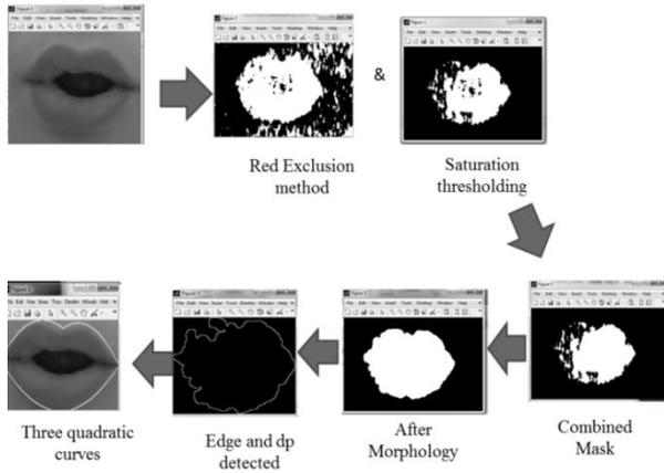
Figure 1: Extraction process of outer lip contours
