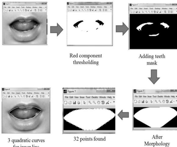
Figure 2: Extraction process of inner lip contours
