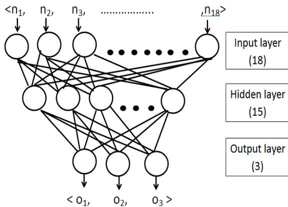
Figure 5: The three layer FeedForward Artificial Neural Network
