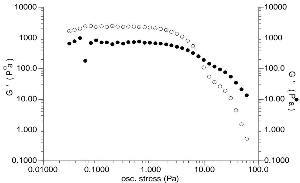
**Figure 2.** Elastic modulus ( $G'$ ), loss modulus ( $G''$ ) versus oscillation stress at 1Hz, 10°C.
