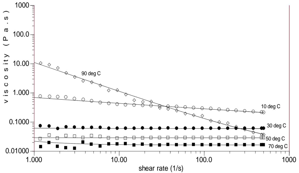
**Figure 1.** Viscosity- shear rate curves of *Moringa oleifera* oil at different temperatures fitted to several rheological models
