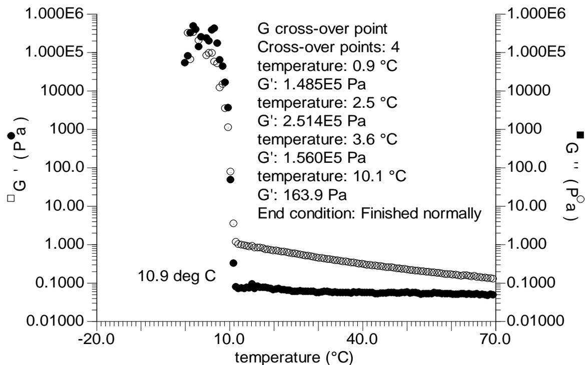
**Figure 3.** Temperature sweep showing elastic modulus ( $G'$ ), loss modulus ( $G''$ ) versus temperature at frequency of 1Hz, oscillation stress of 0.1 Pa
