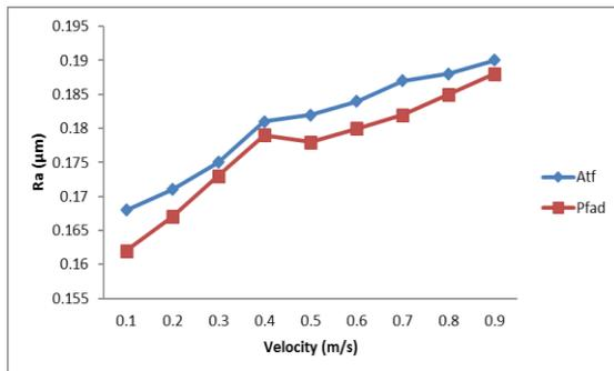
**Figure 6** Surface roughness against velocity at 80°C for ATF and PFAD
