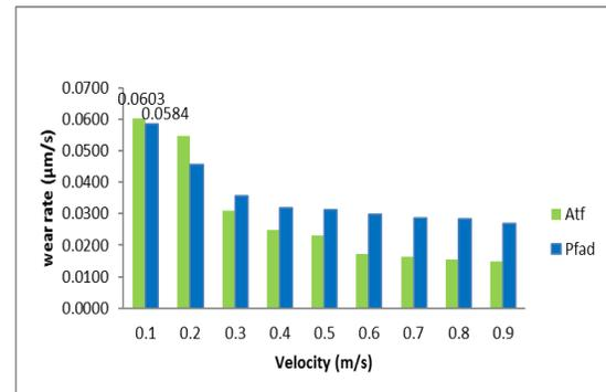
**Figure 5** Wear rate against velocity at temperature 80°C of ATF and PFAD
