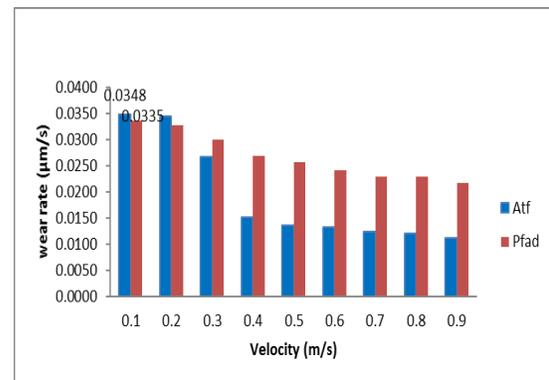
**Figure 4** Wear rate against velocity at temperature 50°C of ATF and PFAD
