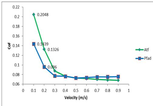
**Figure 2** CoF against velocity at two different temperature 50°C for ATF and PFAD
