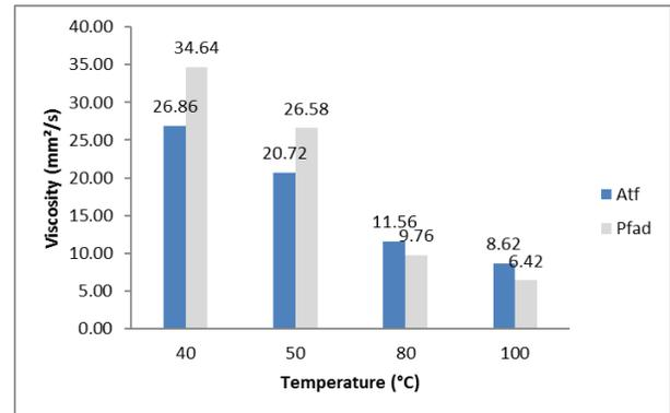
**Figure 1** Viscosity for ATF and PFAD at four different temperatures
