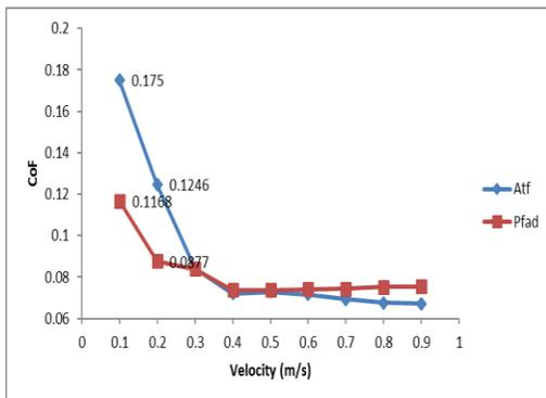
**Figure 3** CoF against velocity at temperature 80°C for ATF and PFAD
