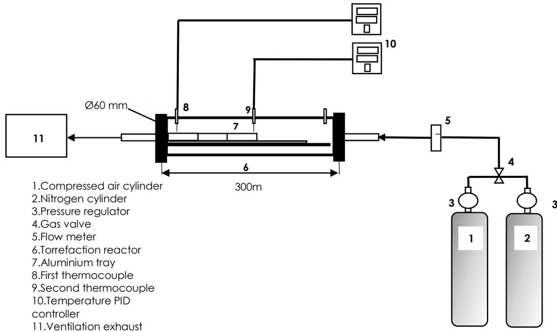
Figure 1 Schematic diagram of setup for torrefaction experiment
