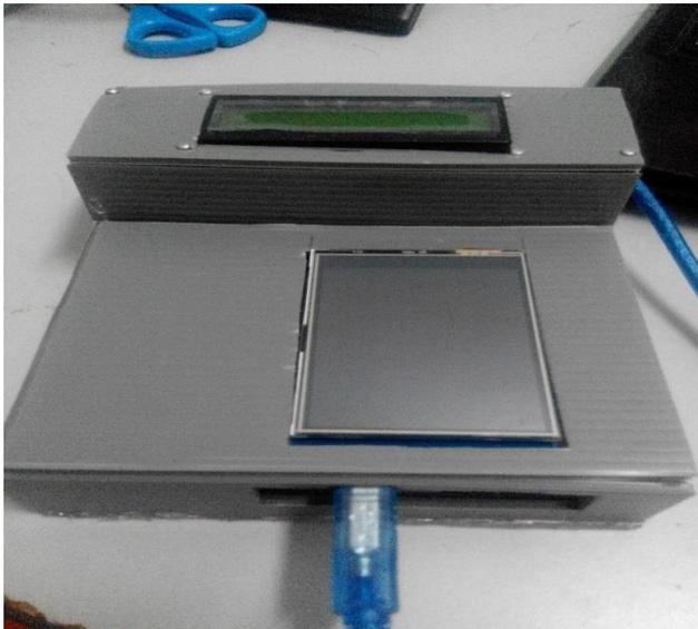
Figure 5 Prototype of the Handwriting Recognition System
