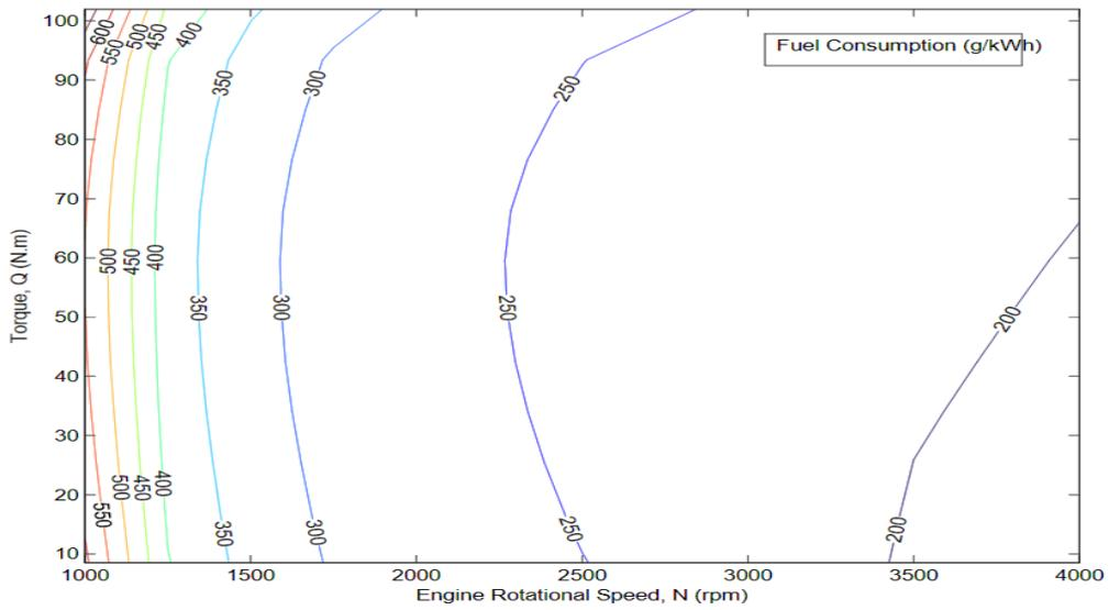
Figure 10 Engine Fuel Consumption Map
