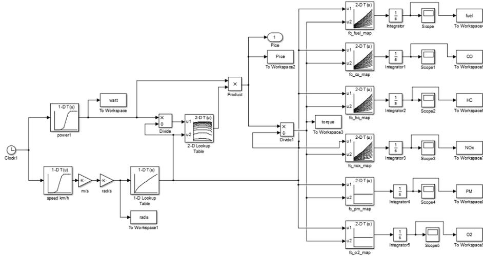
Figure 5 ICE model in MATLAB/SIMULINK environment
