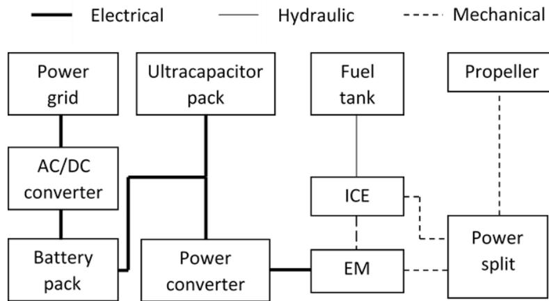
Figure 1 A schematic illustration of PHERB [3-6]
