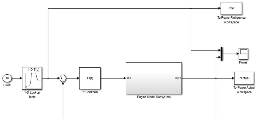
Figure 6 Closed Loop Feedback Control System
