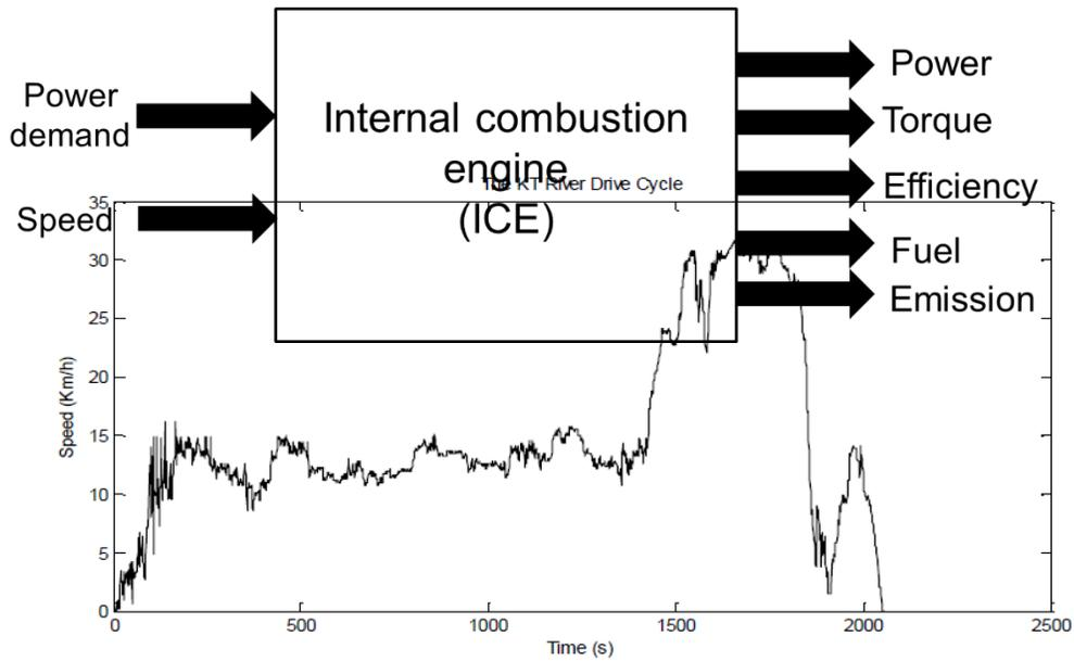
Figure 2 Basic block diagram for ICE
