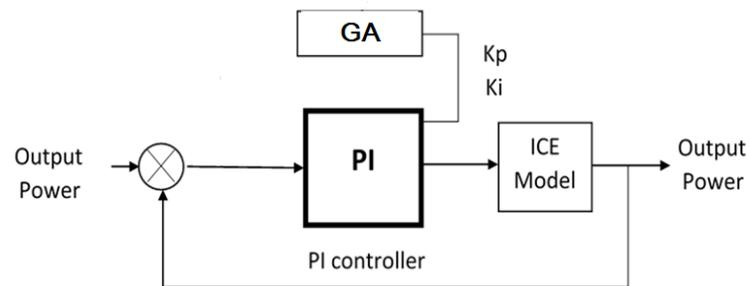
**Figure 7** Block Diagram of PI Controller with Genetic Algorithm
