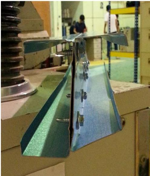
Figure 12 Local buckling failure
