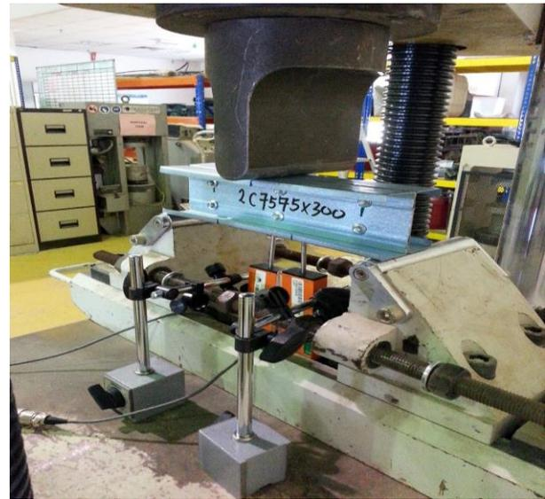
Figure 5 Plain built up beam attached with LVDT
