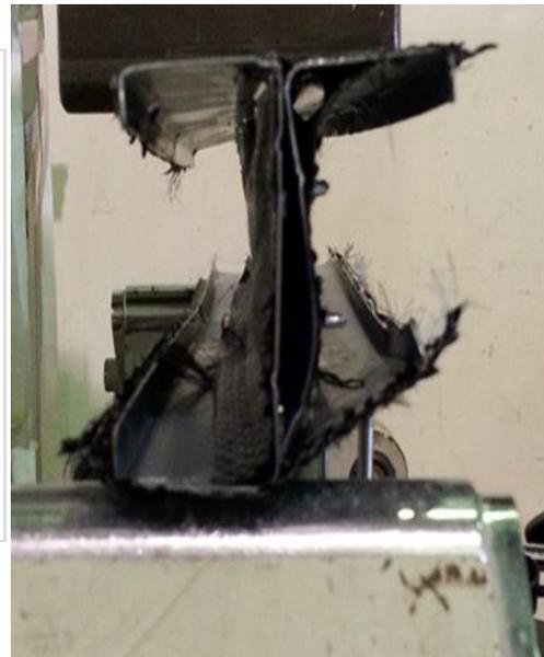
Figure 10 Local buckling failure
