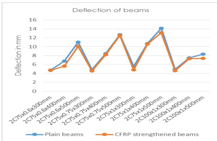
Figure 8 Built up beams deflection measured at mid span
