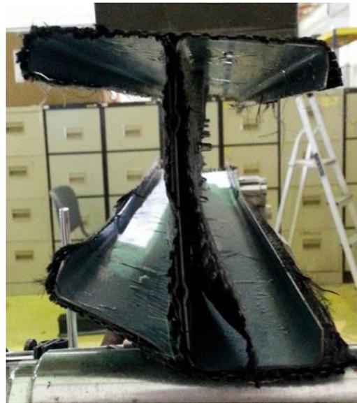
Figure 9 Local buckling failure
