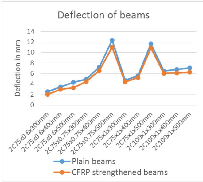
Figure 7 Built up beams deflection measured at one-third span
