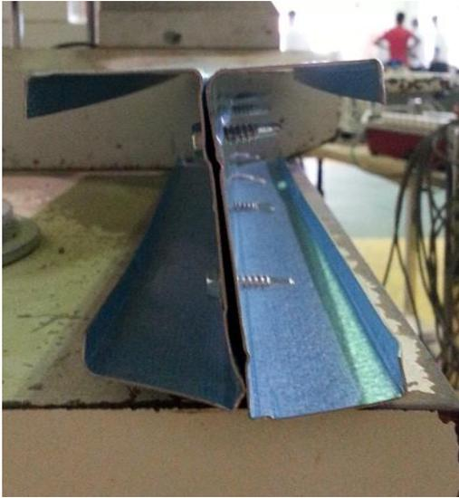
Figure 11 Local buckling failure
