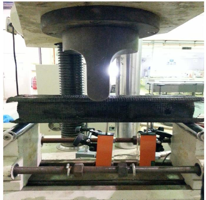
Figure 6 CFRP strengthened built up beam attached with LVDT
