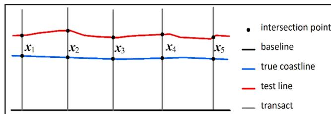
Figure 4: Illustration of baseline approach (Source: USGS, 2014).
