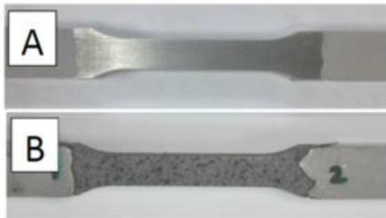
Figure 3 (A) As-received and (B) corrosion pitted tensile specimen
