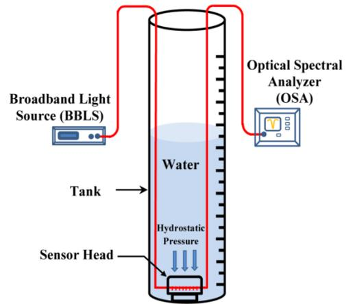
**Figure 4** The experimental set-up for measure water level
