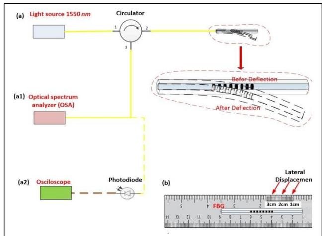
**Figure 7** (a) Experiment set up of tension and curvature effect on FBG. (a1) using (OSA) to retrieve the reflected spectrum data. (a2) using oscilloscope to record the change in the voltage, the discrete lines represents using oscilloscope to record the change in the voltage. (b) Location of applied stress
