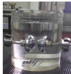
Figure 4: Test cell filled with oil sample.
