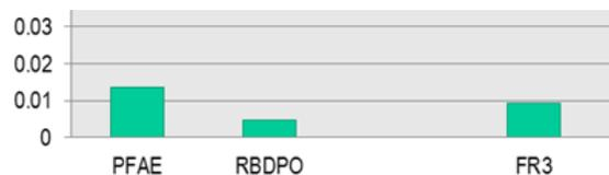
Figure 9: Dissipation factor result for the oil samples
