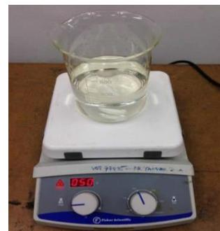
Figure 3: Stirring process in test preparation of the oil sample.
