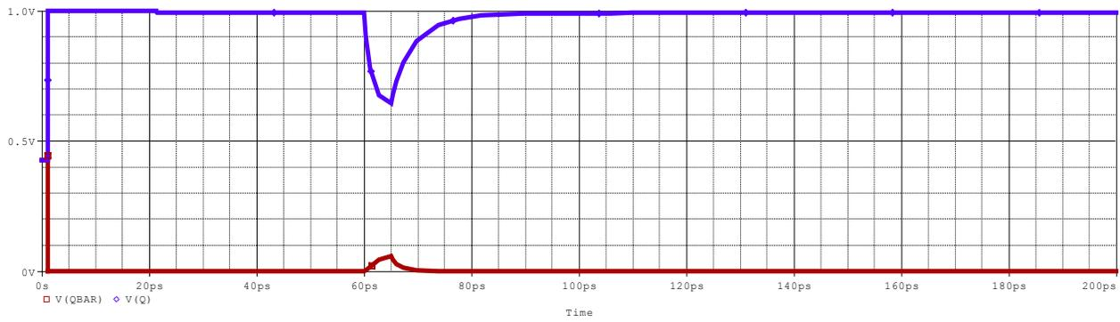
Figure 8: No upset is occurred when the injected current is 0.46mA
