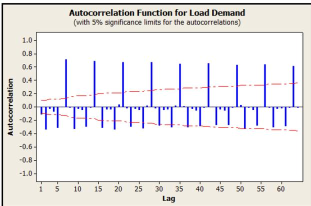
Figure 3: Collelogram for ACF plot
