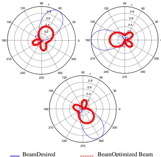
Figure 3: Beam Rotation of 3 Element Array
