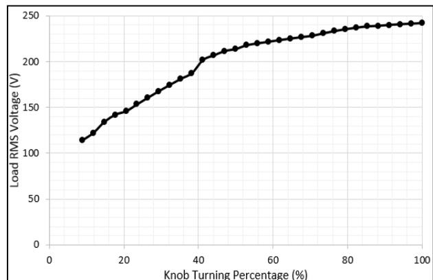
Figure 10: Load RMS Voltage vs Knob Turning Percentage
