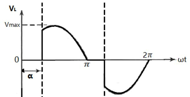
Figure 1: TRIAC Output Voltage Waveform
