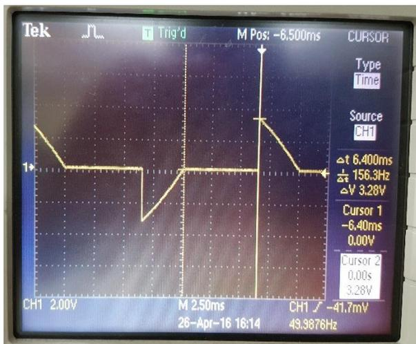
Figure 7: Measuring Exact Delay Time using Oscilloscope
