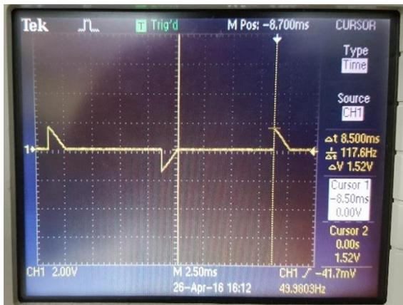
Figure 4: Measuring Exact Delay Time
