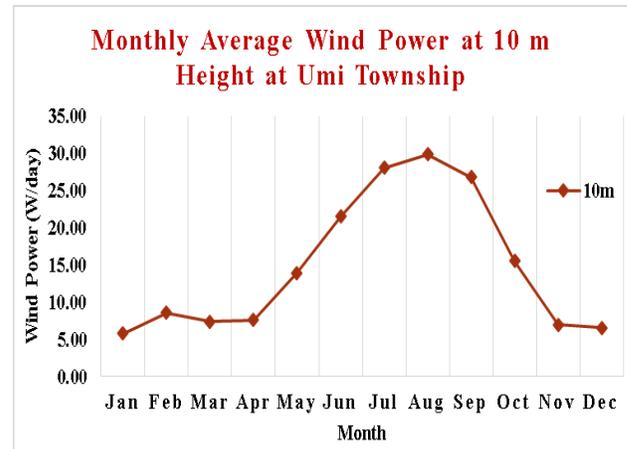
Figure 11: New Umi township site wind power for the 10 m height
