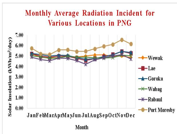
Figure 2: Solar radiation incidents at selected locations in PNG
