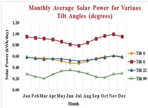
Figure 7: New Umi township solar power at various tilt angles
