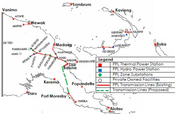
Figure 1: PNG Power Limited electricity supply network, (Source: PPL Planning Department, 2008)
