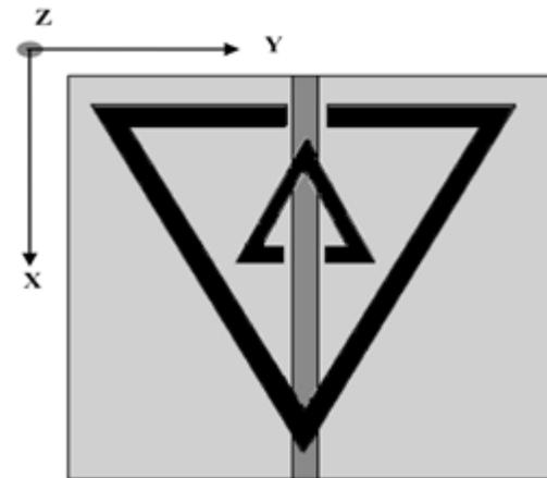
Figure 6: Metamaterials based triangular split ring resonators [28]
