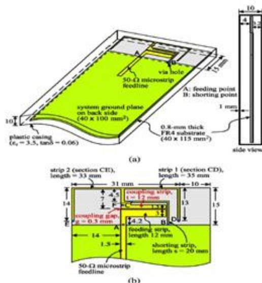
Figure 2: (a) printed PIFA antenna . (b) Dimensions of the PIFA.[15].
