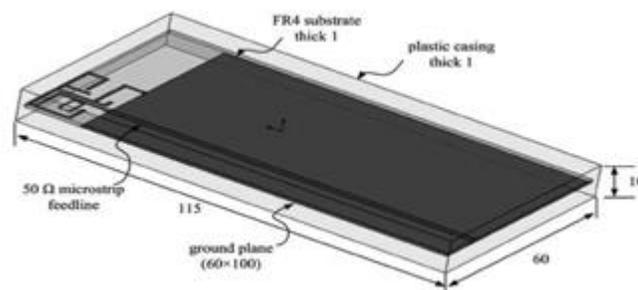
Figure 3: Monopole antenna for octaband mobile application [17].
