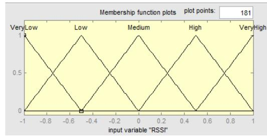
Figure 2: Fuzzy Logic - Triangular Function of Input (RSSI)
