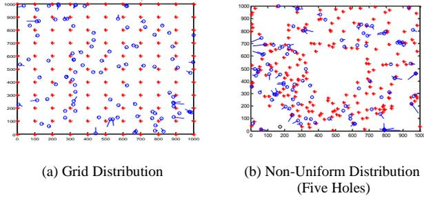
Figure 3: Node Distribution Deployment (cross = anchor; circle = unknown; line = absolute error)
