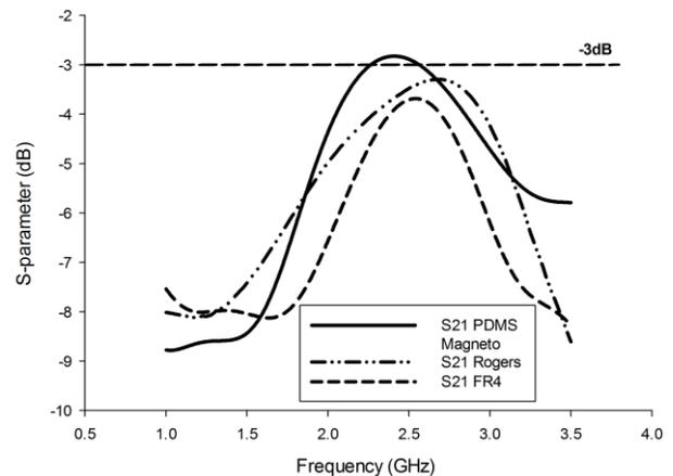
Figure 5: Comparative simulated result for insertion loss (S<sub>21</sub>) performance operates at 2.45 GHz
