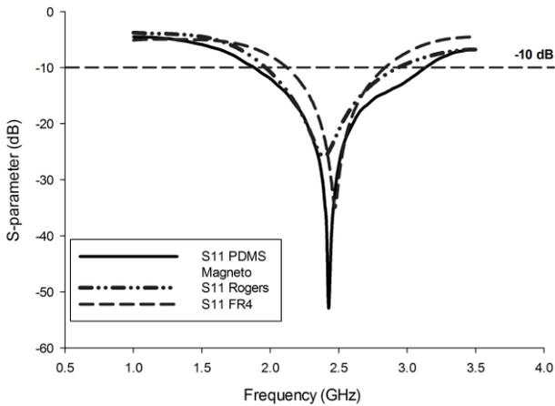
Figure 4: Comparative simulated result for S<sub>11</sub> performance operates at 2.45 GHz
