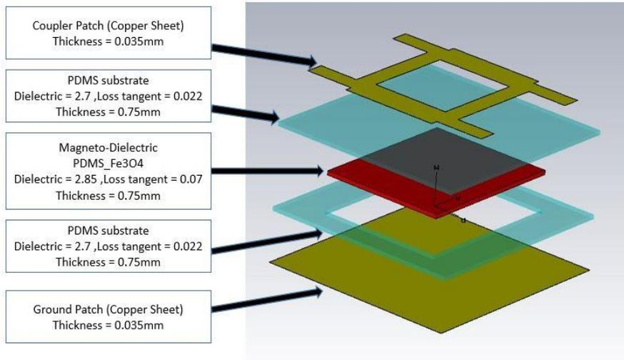
Figure 3: Complete structure layer for branch line coupler on (PDMS-Fe<sub>3</sub>O<sub>4</sub>) substrate
