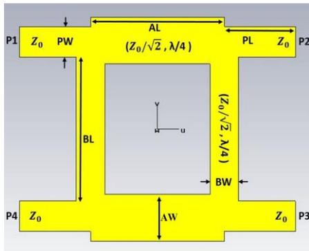
Figure 1: Geometry design of branch line coupler at 2.45 GHz
