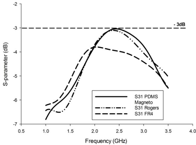
Figure 6: Comparative simulated result for coupling ( $S_{31}$ ) performance operates at 2.45 GHz
