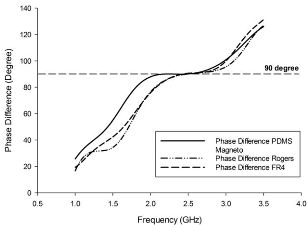
Figure 8: Comparative simulated result for phase difference operates at 2.45 GHz
