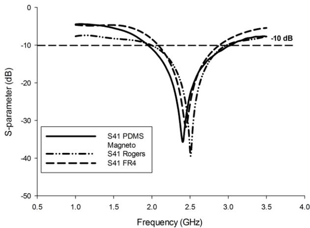
Figure 7: Comparative simulated result for ( $S_{41}$ ) performance operates at 2.45 GHz
