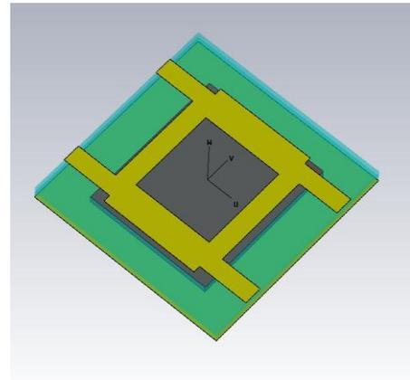
Figure 2: Complete branch line coupler with (PDMS- Fe<sub>3</sub>O<sub>4</sub>) substrate.
