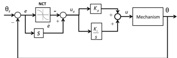
Figure 3: Structure of CM-NCTF controller
