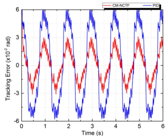
Figure 12: Tracking response to sinusoidal input of 1 Hz, 4 rad
