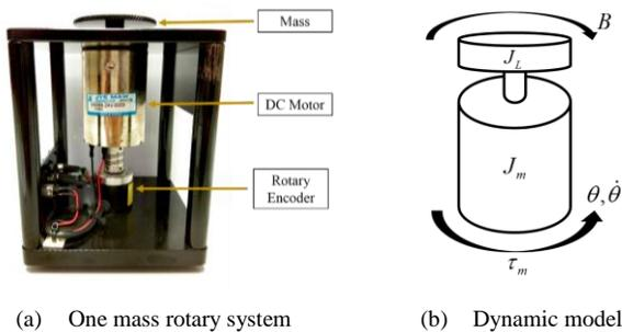
Figure 2: A one mass rotary system and its dynamic
