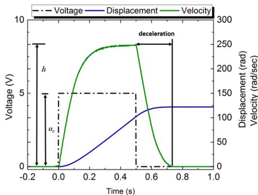
Figure 5: Open loop response with step-wise input
