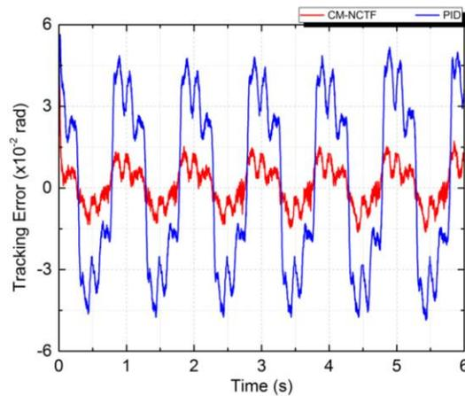
Figure 11: Tracking response to sinusoidal input of 1 Hz, 1 rad
