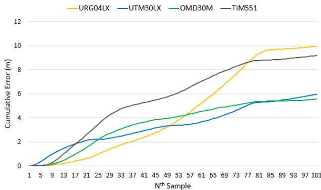
Figure 5: Cumulative error results from each of laser scanners.
