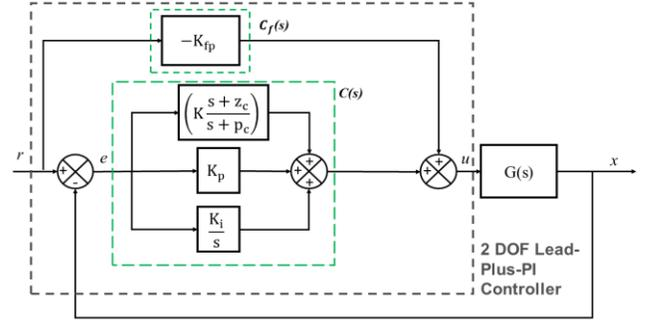
Figure 2: Block diagram of 2-DOF Lead-plus-PI controller
