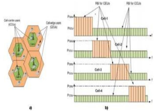
Figure 1: Illustration of the conventional SFR, a) Four adjacent cells with the interior region contains CCUs and the exterior regions contains CEUs, and b) the number of resources and the resource power level in the conventional SFR.
