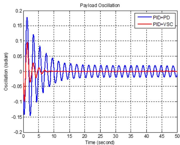
Figure 7: Response of payload oscillation
