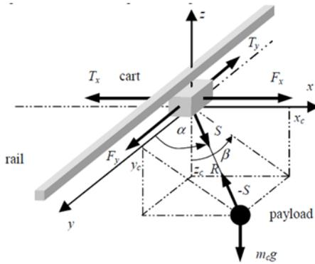
Figure 2: Schematics of 3D gantry crane system
