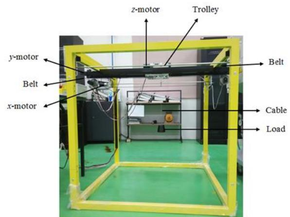
Figure 1: 3D INTECO Crane System
