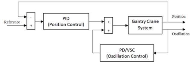
Figure 3: Block diagram of control structure in gantry crane system
