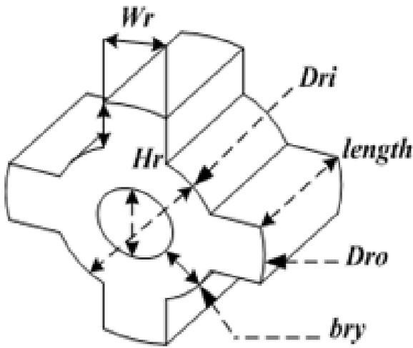
Figure 2: Basic geometry of SRM rotor
