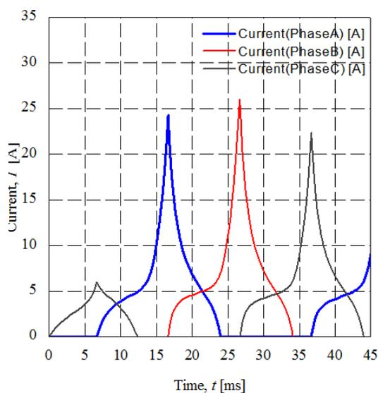
Figure 11: Winding current while inductance descends
