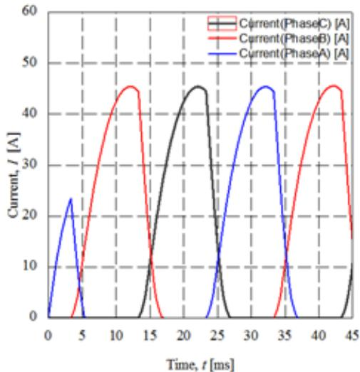
Figure 7: Winding current before inductance ascends
