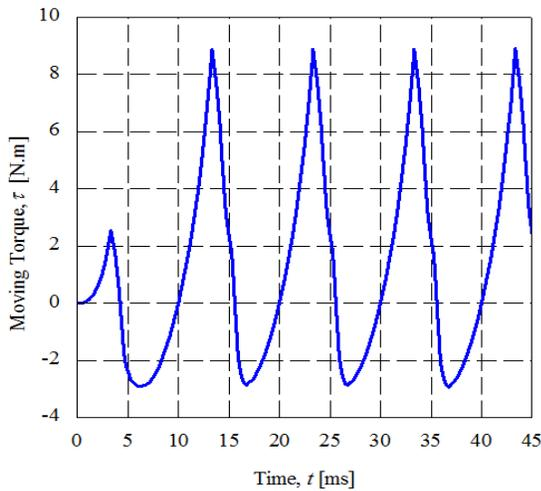
Figure 6: Torque production before inductance ascends
