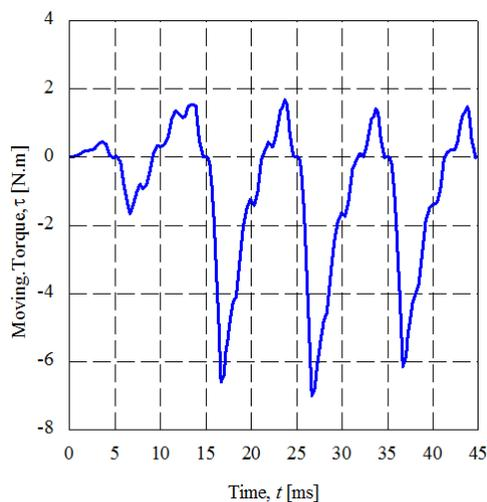
Figure 10: Torque production after inductance descends
