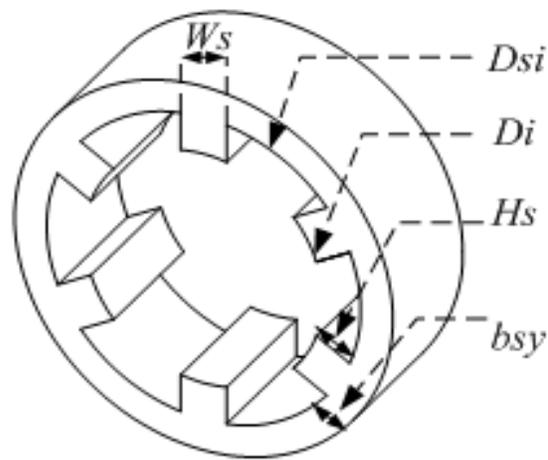
Figure 1: Basic geometry of SRM stator
