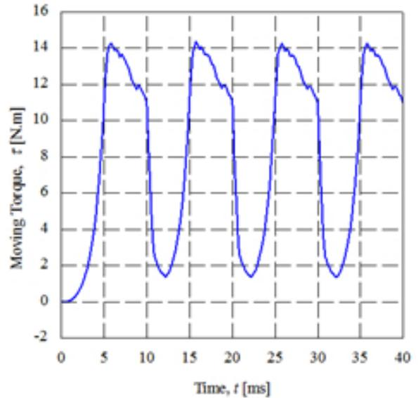
Figure 8: Torque production while inductance ascends
