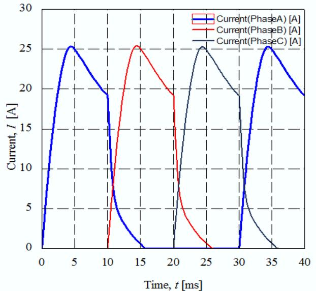
Figure 9: Winding current while inductance ascends
