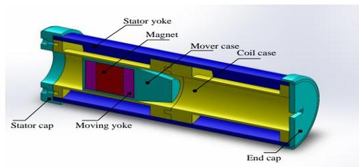
Figure 10: Cross-sectional view of linear actuator.
