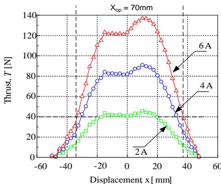
Figure 8: Performance current characteristic.
