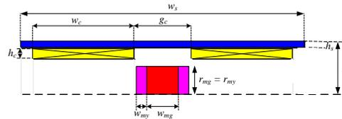
Figure 5: The parameters in structure modeling of the linear actuator
