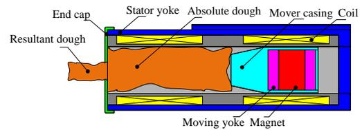
Figure 1: The slot-less linear actuator.
