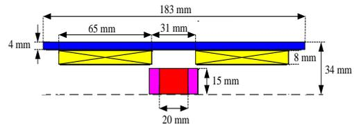
Figure 9: Full specification of chosen linear actuator.
