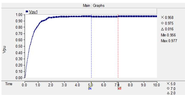
Figure 8: Simulation with Fault with 6-Pulse STATCOM Single Phase to Ground.
