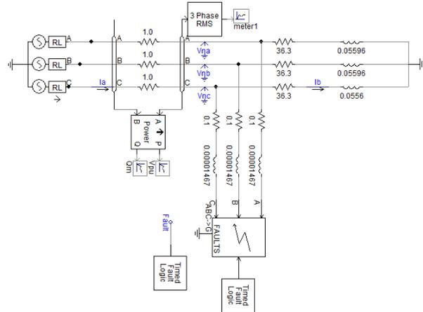
Figure 4: Simulation System with Fault without STATCOM
