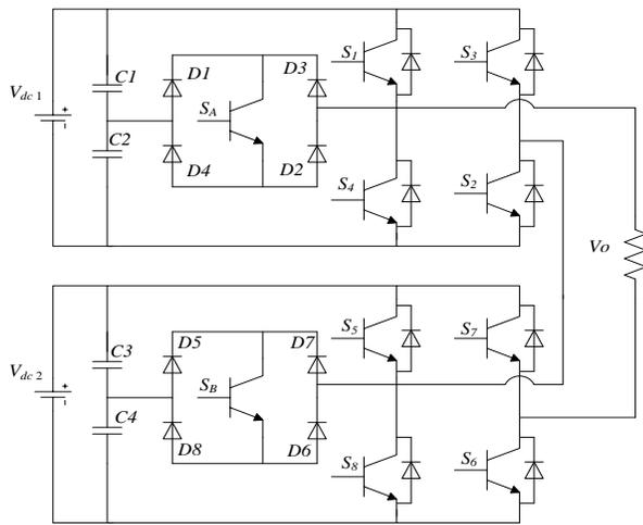
Figure 7: Hybridised cascaded H-bridge (HCHB) multilevel inverter
