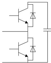
Figure 8: Single modular multilevel converter (MMC) cell
