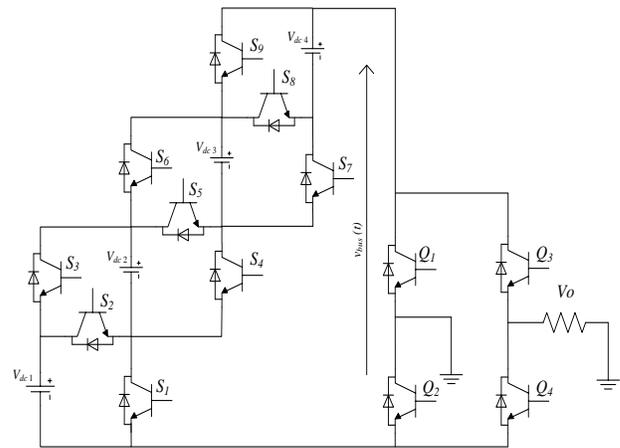
Figure 10: Switched series/parallel sources (SSPS)-based multilevel inverter
