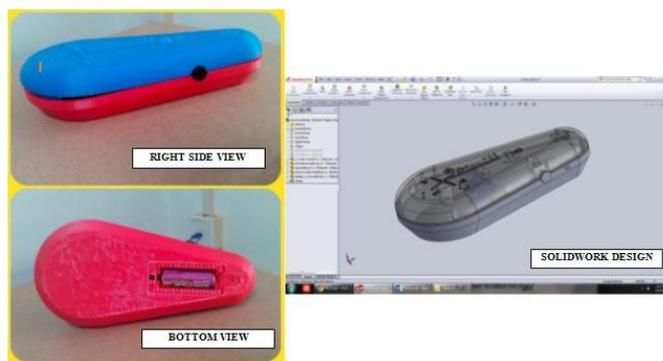
Figure 3: The second casing design
