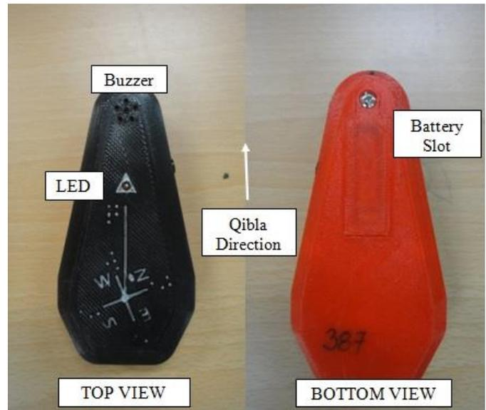
Figure 6: Qibla compass final design
