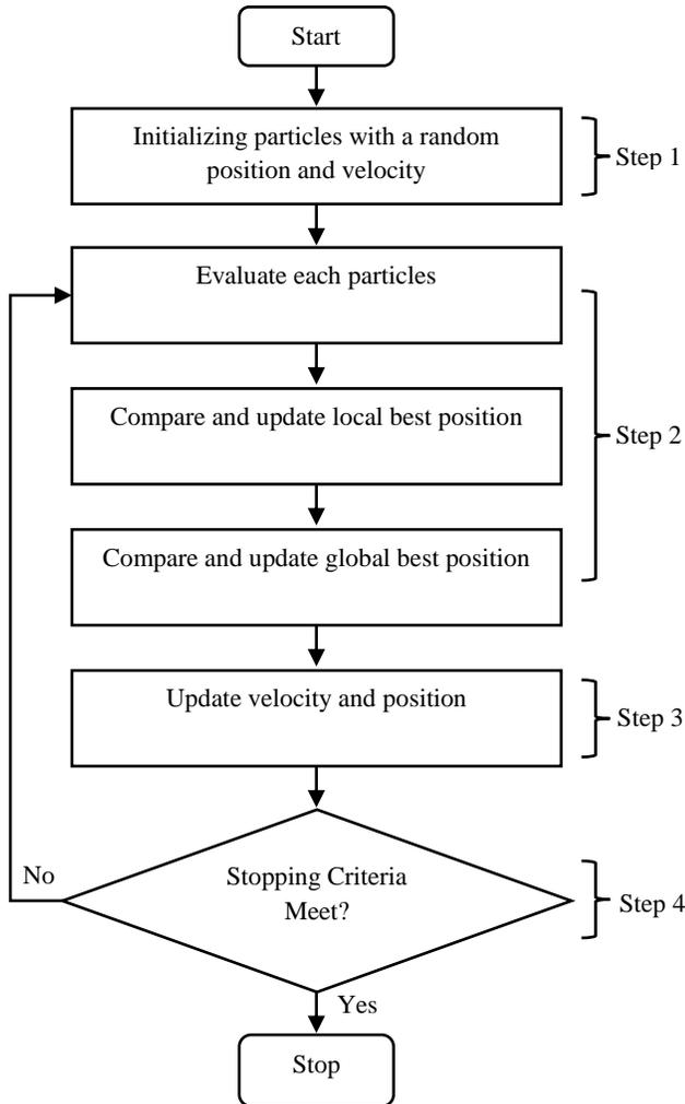
Figure 4: The execution process of PSO algorithm
