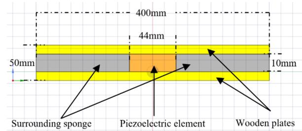
Figure 4: Schematic diagram of a human single step piezoelectric generator prototype
