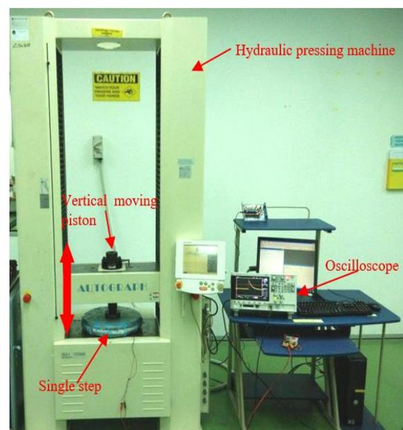
Figure 5: Experimental set-up to measure voltage generation of the single step piezoelectric generator prototype (labelled as ‘single step’)
