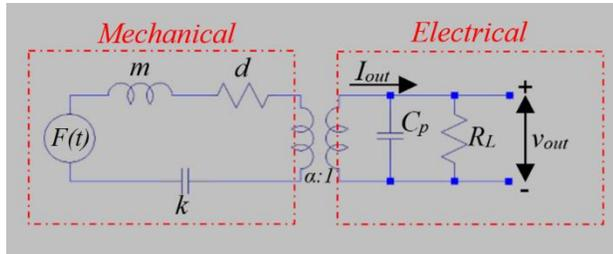
Figure 3: The equivalent circuitry of the piezoelectric harvester.
