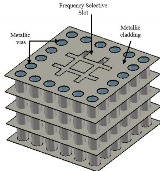
Figure 2: FSS using cascading SIW cavities [18]
