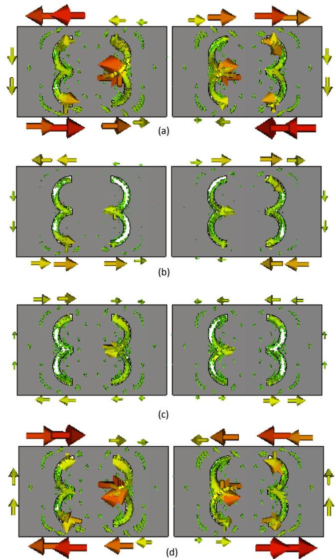
Figure 5: Surface current of upper part of the parasitic element with three-shaped slot at the patch antenna for resonant frequency of 1.8 GHz at different phase, (a) phase =  $0^\circ$ , (b) phase =  $90^\circ$  (c) phase =  $135^\circ$ , (d) phase =  $180^\circ$
