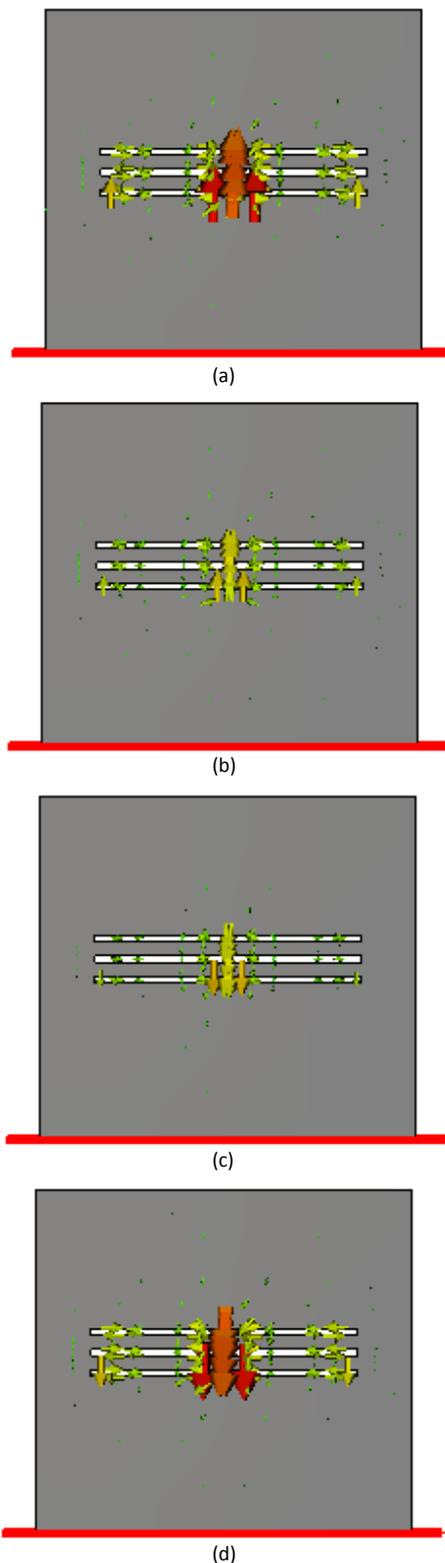
Figure 6: Surface current of the ground plane patch antenna for resonant frequency of 1.8 GHz at different phase, (a) phase =  $0^\circ$ , (b) phase =  $90^\circ$  (c) phase =  $135^\circ$ , (d) phase =  $180^\circ$
