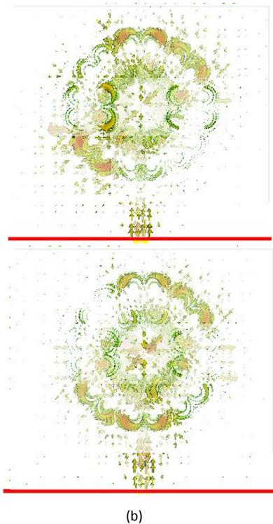
Figure 4: Surface current of the dual band antenna, (a) first resonant frequency at 1.8 GHz, current phase =  $0^\circ$  and  $90^\circ$  (b) second resonant frequency at 5.2 GHz, current phase =  $0^\circ$  and  $90^\circ$
