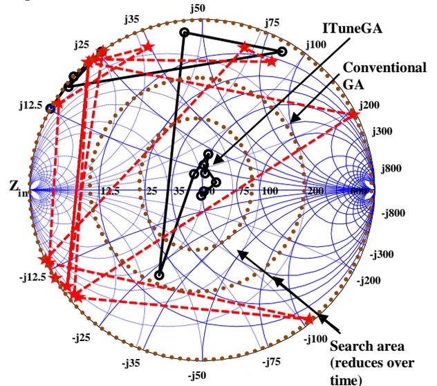
Figure 5: Convergence of ITuneGA and the conventional GA based on complex input impedances in Smith chart
