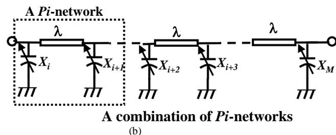
Figure 2: (a) Block diagrams of an adaptive impedance tuning network and their parameters (b) a  $Pi$ -network topology
