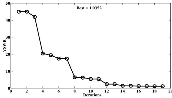
Figure 8: Convergence of ITuneGA based on VSWR over number of iterations for the impedance tuner with four tuning elements
