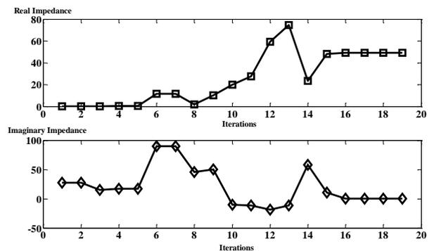
Figure 6: Convergence of ITuneGA based on real and imaginary parts of input impedance over number of iterations
