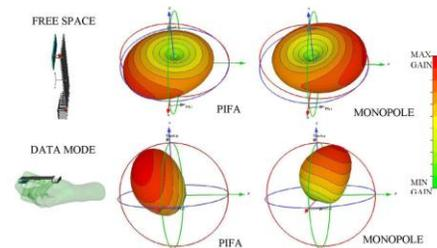
Figure 1: Effect of human hand (in data mode position) to the antenna gain patterns at 881.5MHz frequency [9]
