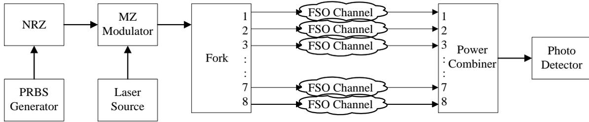
Figure 1: TXs/RXs FSO link simulation layout.
