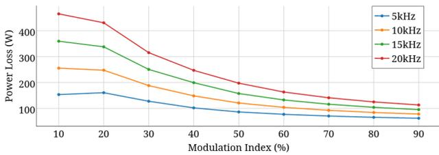
Figure 4: Switch power losses in 300V input voltage
