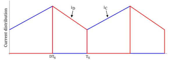
Figure 2: Currents distribution for the buck converter
