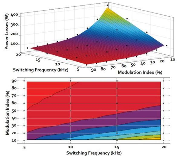
Figure 6: 3D and contour plot of the power losses at 8kW output power
