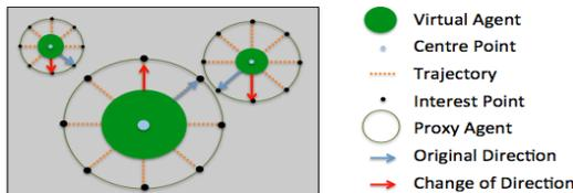
Figure 3: Illustrations of the parameters applied in a proxy agent.
