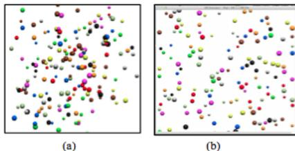
Figure 4: Result of simulation of virtual agents (a) Without collision avoidance and (b) With collision avoidance with the aid of proxy agent
