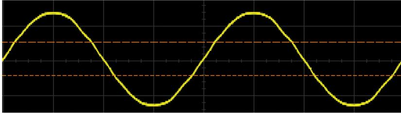
Figure 4. Measured AC source voltage,  $v_{ac}$  (scale: 50 V/div).
