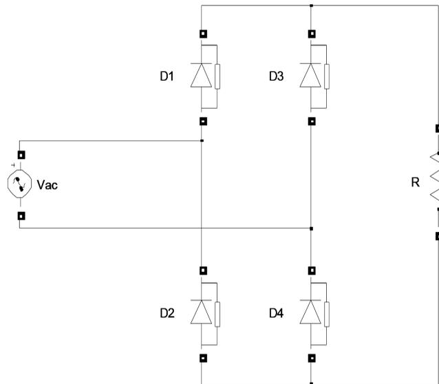
Figure 1. Single phase diode bridge rectifier circuit model.
