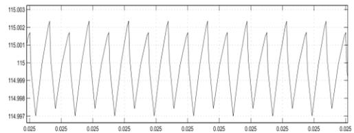
c) Converter Output Voltage Ripple = 115.0025V - 114.9975V = 0.005Volt
