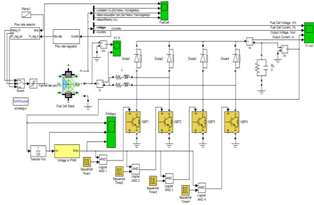
Figure 11 Simulation Model of the Conventional MDIBC
