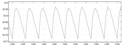
a) Fuel Cell Input Voltage Ripple = 60.195V - 60.173V = 0.022Volt
