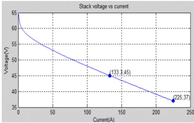
Figure 14 6kW PEMFC V-I curve
