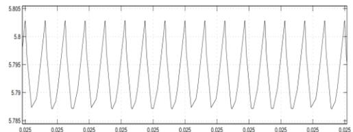
b) Fuel Cell Input Current Ripple = 5.803A - 5.787A = 0.016Amp
