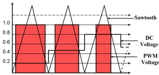
**Figure 10** Creating a PWM Signal by comparing two waveforms
