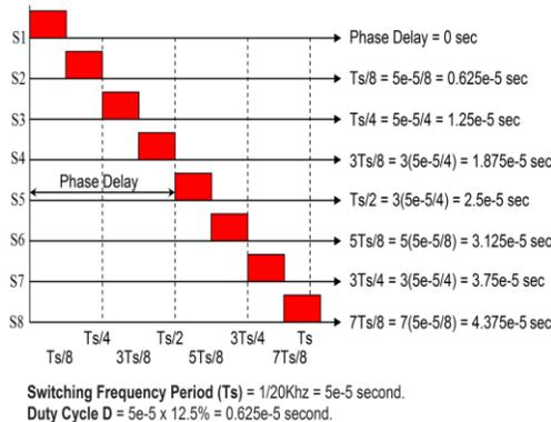
Figure 7 Sequence of the Improved MDIBC input signals
