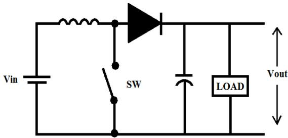
Figure 2 Conventional boost converter
