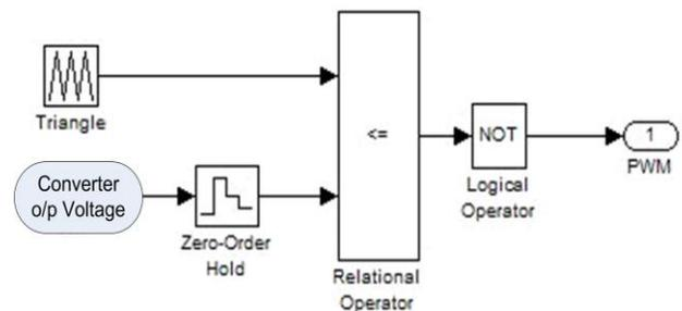
Figure 9 Simulink Model for PWM Generator
