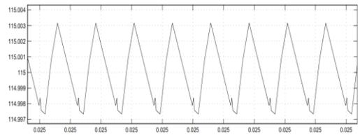
c) Converter Output Voltage Ripple = 115.0032V - 114.9974V = 0.006Volt
