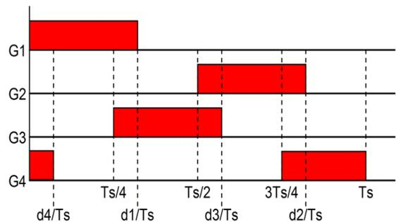
Figure 5 Overlap phase-shift interleaved control
