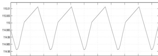
c) Converter Output Voltage Ripple = 115.01V - 114.98V = 0.03Volt
