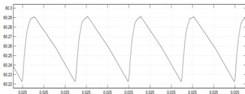
a) Fuel Cell Input Voltage Ripple = 60.29V - 60.22V = 0.07Volt
