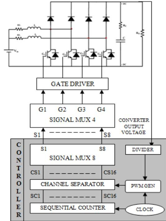
Figure 8 Block Diagram of Proposed Novel Multiplex Controller
