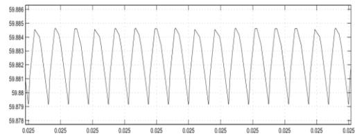
a) Fuel Cell Input Voltage Ripple = 59.8845V - 59.8792V = 0.0053Volt
