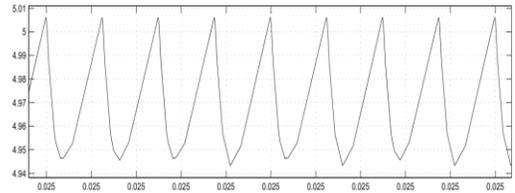
b) Fuel Cell Input Current Ripple = 5.006.A - 4.944A = 0.062Amp
