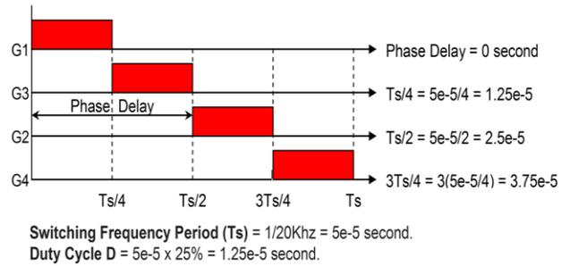
Figure 4 Sequences of the gate signals to provide double ripple frequency and to achieve the interleaved control
