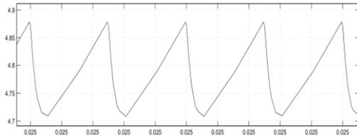
b) Fuel Cell Input Current Ripple = 4.87A - 4.71A = 0.16Amp
