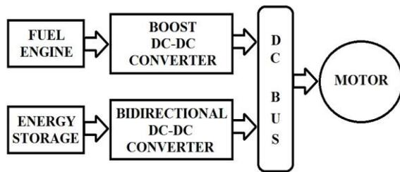
**Figure 1** Power supply system of fuel cell electric vehicle
