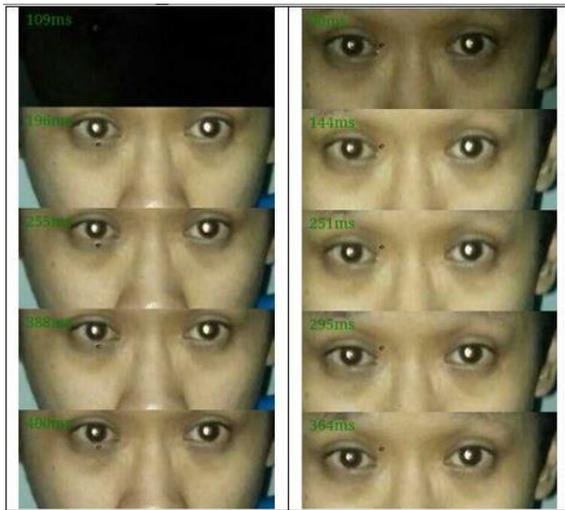
Figure 16 Flash Timing Test, photos are taken consecutive with set timer. However, each shots results in different timing due to delay in mobile phone
