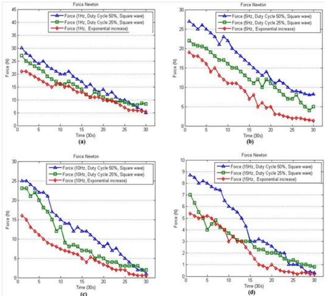
Figure 4 Muscle forces versus time for the frequency (a) 1 Hz, (b) 5 Hz, (c) 10 Hz and (d) 15 Hz for the 50 mA current amplitude
