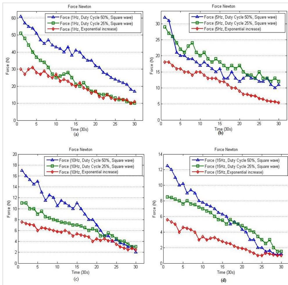
**Figure 6** Muscle forces versus time for the frequency (a) 1 Hz, (b) 5 Hz, (c) 10 Hz and (d) 15 Hz for the 100 mA current amplitude
