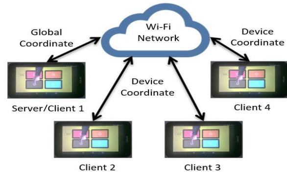
Figure 2 Client-server architecture for mobiTop system
