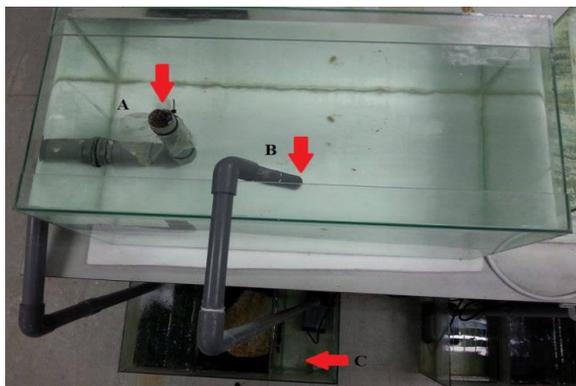
**Figure 3** Glass aquarium used for observing the behaviour of phyllidiid species: A. The outlet; B. The inlet of filtered sea water; C. Filtration system
