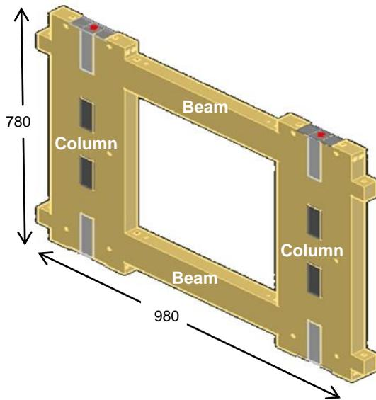
Figure 1(c) Conventional Sub Frame Model
