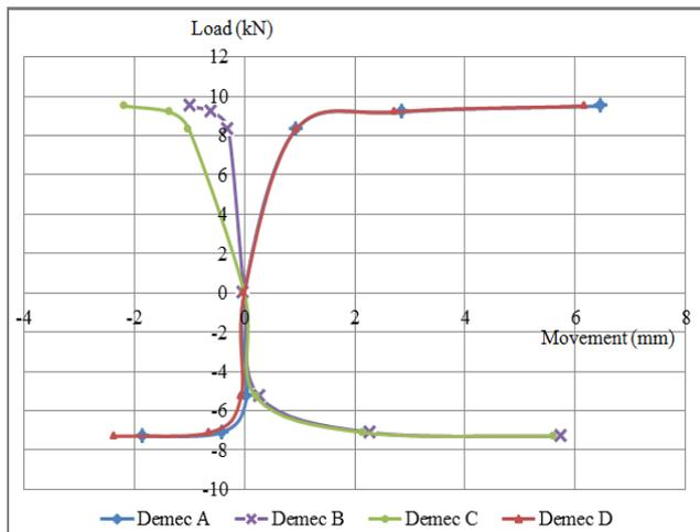
Figure 8 Load and Demec Movement of Conventional Sub-system
